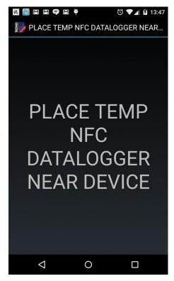
Bring the NFC Temp closer to the NFC antenna of your phone (attention! Each phone has the NFC antenna positioned at different points, usually on the back) and do not move it away until the screen turns blue to green. If it turns red, repeat the operation, being careful not to move the logger.
